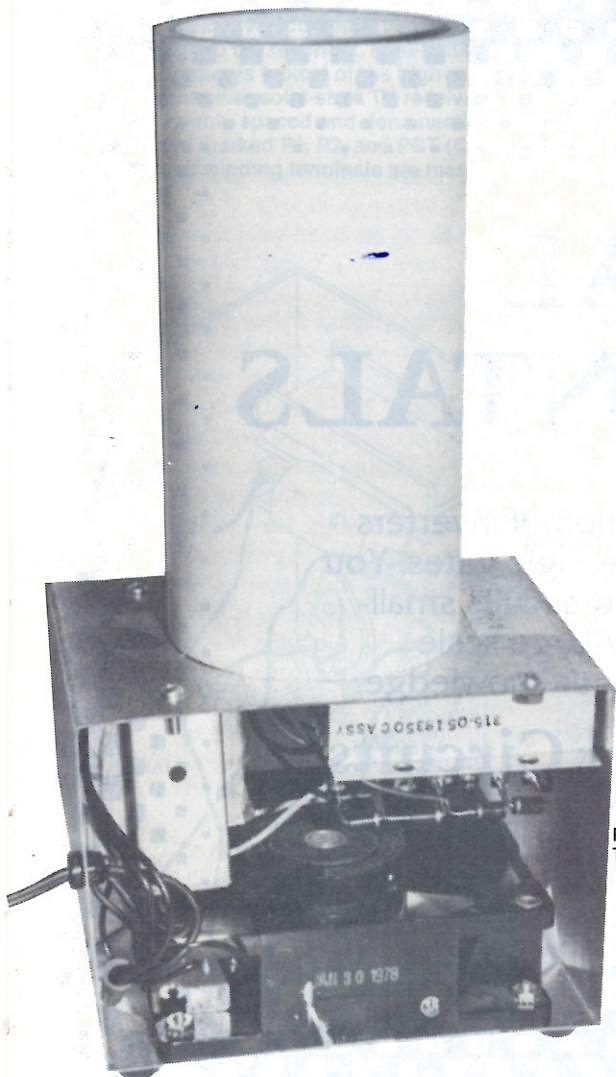
A rear view of the bracket assembly with the electrical parts in place and the PVC extender tube (EXT1) installed. The 1 \frac{3}{4} -inch hole in the extender tube is not visible in this view.
