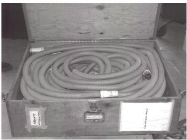
Connect with 7 tubes each of the 7 exits of the windmachine with one yellow pillow.
