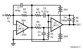
This circuit shows how two amplifiers can be cascaded to double output swing. The advantage over the bridge is that the output can be increased with any number of stages, although separate supplies are required for each.
