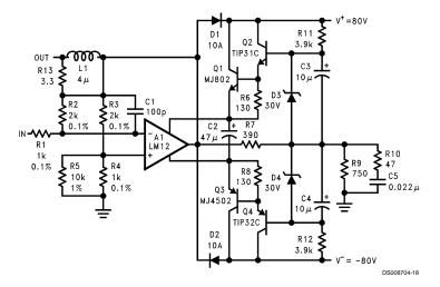
Discrete transistors can be used to increase output drive to  $\pm$ 70V at  $\pm$ 10A as shown above. With proper thermal design, the IC will provide safe-area protection for the external transistors. Voltage gain is about thirty.
