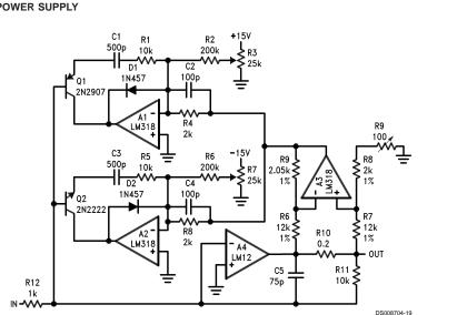
Note: Supply voltages for the LM318s are ±15V
