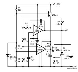
Dual supplies are not required to use an op amp as a voltage regulator if zero output is not required. This 4V to 50V regulator operates from a single supply. Should the op amp not be able to absorb enough energy to control an overvoltage condition, a SCR will crowbar the output.
