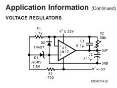
An op amp can be used as a positive or negative regulator. Unlike most regulators, it can sink current to absorb energy dumped back into the output. This positive regulator has a 0-50V output range.
