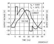
Should the power ratings of the LM12 be exceeded, dynamic safe-area protection is activated. Waveforms with this power limiting are shown for the LM12 driving ±26V at 30 Hz into 3 $\Omega$  in series with 24 mH ( $\theta$  = 45<sup>°</sup>). With an inductive load, the output clamps to the supplies in power limit, as above. With resistive loads, the output voltage drops in limit. Behavior with more complex RCL loads is between these extremes.
