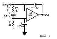
Extending input compensation to the integrator connection is shown here. Both the follower and this integrator will handle 1  $\mu$ F capacitive loading without LR output isolation.
