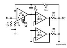
Output drive beyond the capability of one power amplifier can be provided as shown here. The power op amps are wired as followers and connected in parallel with the outputs coupled through equalization resistors. A standard, high-voltage op amp is used to provide voltage gain. Overall feedback compensates for the voltage dropped across the equalization resistors.
