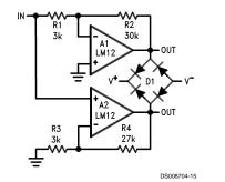
The voltage swing delivered to the load can be doubled by using the bridge connection shown here. Output clamping to the supplies can be provided by using a bridge-rectifier assembly.
