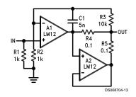
This connection allows increased output capability without requiring a separate control amplifier. The output buffer,  $A_2$ , provides load current through  $R_5$  equal to that supplied by the main amplifier,  $A_1$ , through  $R_4$ . Again, more output buffers can be added.
