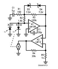
This position servo uses an op amp to develop the rate signal electrically instead of using a tachometer. In high-performance servos, rate signals must be developed with large error signals well beyond saturation of the motor drive. Using a separate op amp with a feedback clamp allows the rate signal to be developed properly with position errors more than an order of magnitude beyond the loop-saturation level as long as the photodiode sensors are positioned with this in mind.
