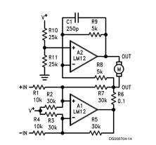
Although op amps are usually operated from dual supplies, single-supply operation is practical. This bridge amplifier supplies bi-directional current drive to a servo motor while operating from a single positive supply. The output is easily converted to voltage drive by shorting  $R_6$  and connecting  $R_7$  to the output of  $A_9$ , rather than  $A_1$ .
