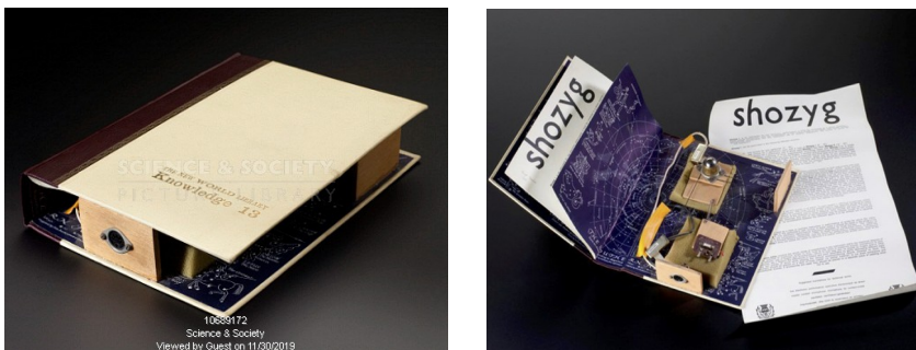
Fig.1.8.1. Shozyg I (1968) - self-built electro-acoustic musical instrument by Hugh Davies. © Science Museum/Science & Society Picture Library. For an audio example go to: https://sounds.bl.uk/Classical-music/Hugh-Davies-experimental-music/026M-C1193X0051XX-0001V0 [last access: 23/05/2021].
