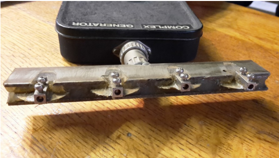
Fig.1.6.1 Holosound component: four piezos encapsulated in silicon with their preamplifier in the black box.
