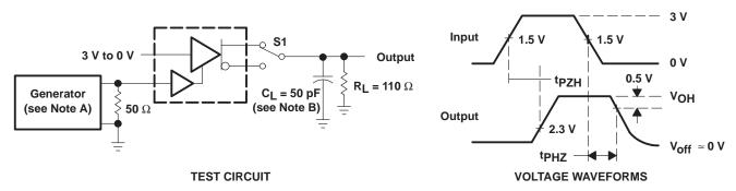
NOTES: A. The input pulse is supplied by a generator having the following characteristics: PRR  $\leq$  1 MHz, duty cycle = 50%,  $t_f \leq$  5 ns,  $Z_O = 50 \ \Omega$ .
