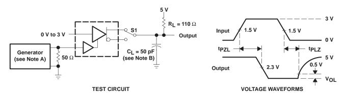
NOTES: A. The input pulse is supplied by a generator having the following characteristics: PRR  $\leq$  1 MHz, duty cycle = 50%,  $t_f \leq$  5 ns,  $Z_O = 50 \ \Omega$ .
