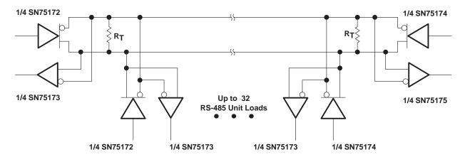
NOTE: The line length should be terminated at both ends in its characteristic impedance (R<sub>T</sub> = Z<sub>O</sub>). Stub lengths off the main line should be kept as short as possible.
