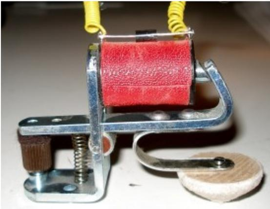
Thanks to these valves, we obtained velocity sensitivity for each individual note as well as individual key pressure modulation (note aftertouch). The sizing of the pallet valves with conical pads is given in the table above. These sizes were calculated such that for a given solenoid trajectory (5 to 10mm) and orifice, flow regulation is optimal. We designed software to calculate the frustum shaped apertures based on the following geometric considerations<sup>3</sup>:
