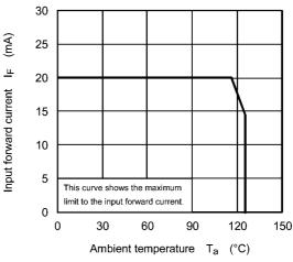
Fig. 12.2.2 I<sub>F</sub> - T<sub>a</sub>
