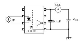
Fig. 12.1.4 I<sub>CCL</sub> Test Circuit
