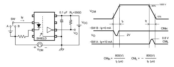
Fig. 12.1.6 Common-Mode Transient Immunity Test Circuit and Waveform
