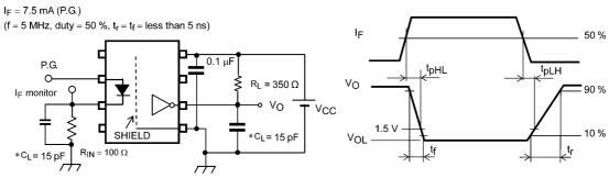
\*CL: includes probe and stray wiring capacitance.
