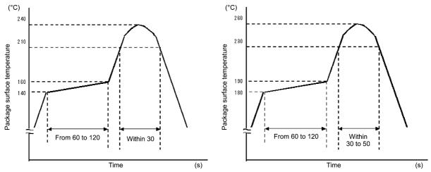
Fig. 13.1.1 An Example of a Temperature Profile Fig. 13.1.2 An Example of a Temperature Profile When Sn-Pb Eutectic Solder Is Used When Lead(Pb)-Free Solder Is Used
