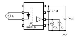
Fig. 12.1.2 V<sub>OL</sub> Test Circuit
